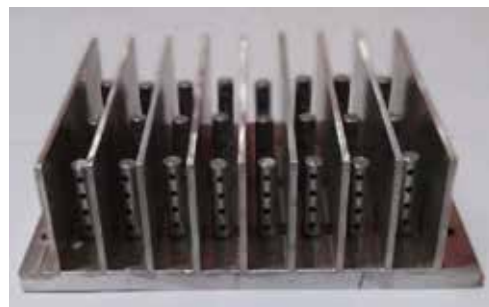
Fig.2 b) Height of pin 35 mm with four perforations
