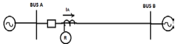
Fig. 3 Basic principle of distance protection
