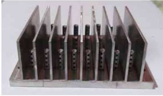
Fig. 2 c) Height of pin 25 mm with four perforations
