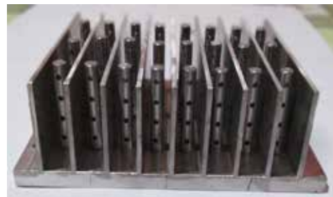
Fig.2 a) Height of pin 50 mm with four perforations
